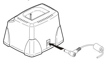
The Power LED is lit when the charger is set up and plugged in.
